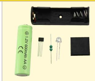
This soldering kit contains all the parts needed to build a solar-powered night light. The components provided can be simply soldered together with a little bit of solder. The circuit is already built and ready for use.
